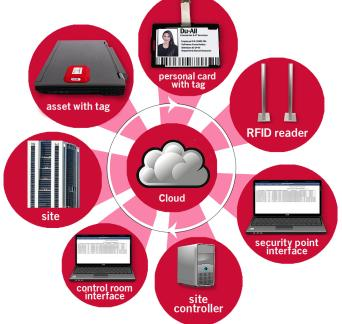
• RFID controllers are installed at the exits and throughout the building. These controllers receive the signals from the various active tags. The range of the controller is between 30 and 100m and depends on the building layout. The messages received from tags can contain the following information: tag ID, battery level, tamper alert, movement detection and location ID.
